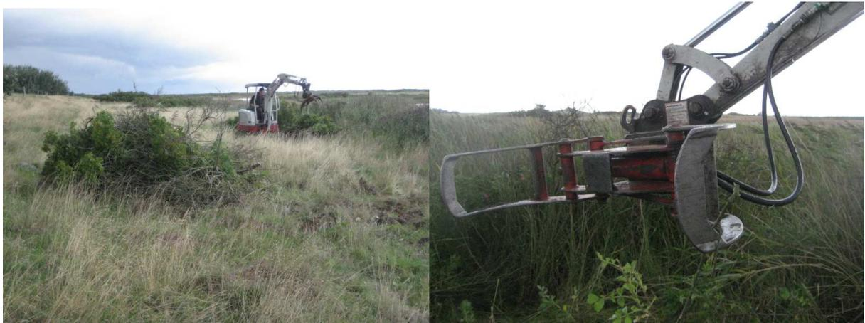
*Removal of Rosa rugosa with roots using a small digging machine equipped with a special tool.*
